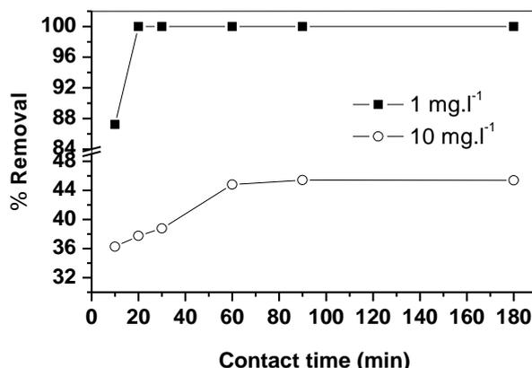
**Figure 7:** Effect of contact time on the removal of rhodamine B, 0.1 g of graphite from spent LIBs anode, 25 mL of RB solution, temperature 25°C.
