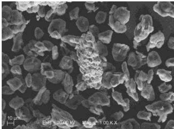
**Figure 3:** Scanning electron micrographs of graphite from spent lithium-ion batteries (LIBs) anode.
