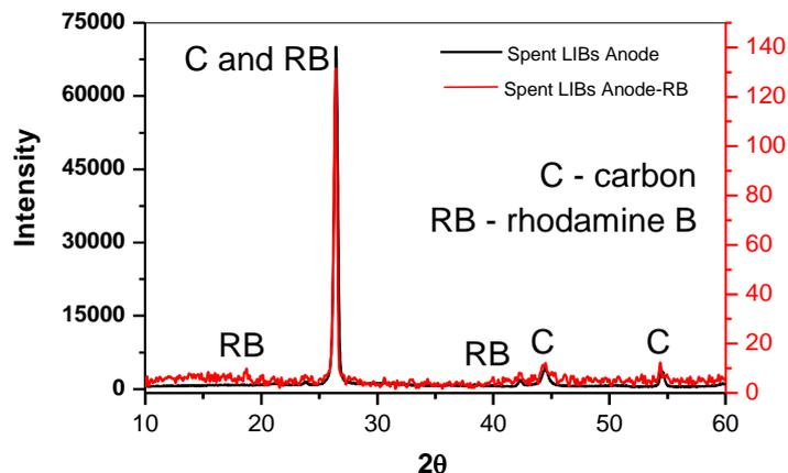
**Figure 1:** XRD patterns of graphite anode active materials from a spent lithium-ion batteries (LIBs) and after adsorbed by Rhodamine B.
