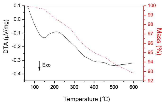
**Figure 2:** The thermogravimetric behavior of the graphite from spent LIBs anode.
