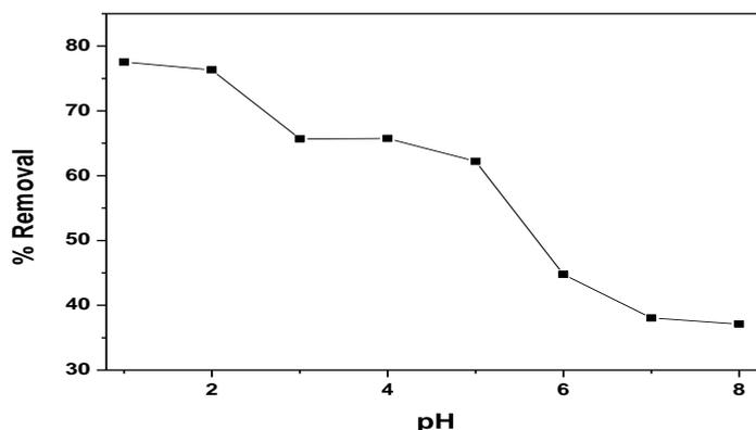
**Figure 8:** Effect of pH on the removal of RB by graphite from spent LIBs anode: 0.1 g of spent LIBs anode, 25 ml of solution, temperature 25°C.
