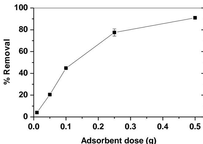
Figure 10: Effect of graphite from spent LIBs anode dosage on the removal of RB, 25 mL of solutions, contact time 60 min, temperature 25°C.
