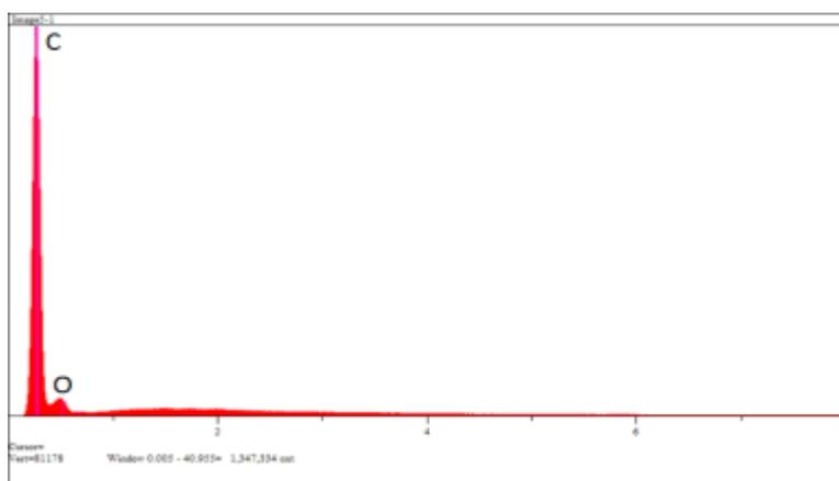
**Figure 4:** Energy Dispersion X-ray (EDX) spectrum of graphite from spent LIBs anode.
