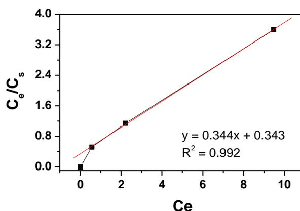
Figure 11: Langmuir adsorption isotherm.
