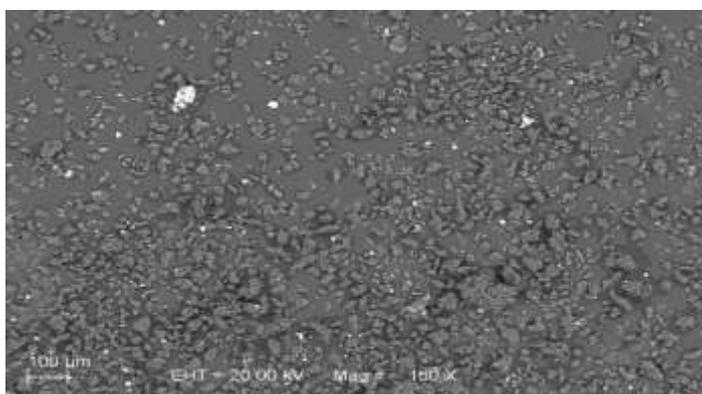
**Figure 5:** SEM images of Rhodamine B on the surface of the graphite from spent LIBs anode.
