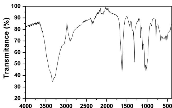
**Figure 6:** Infrared spectrum of the graphite after rhodamine B adsorption.
